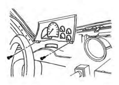
4. Finally, disconnect the instrument cluster electrical connection.
