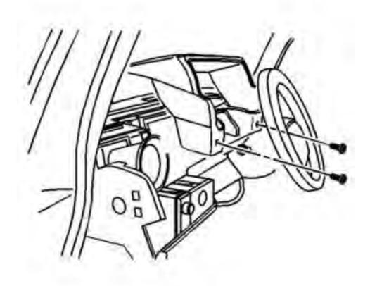
3. Now, remove the screws from the instrument cluster
