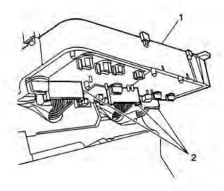
5. Disconnect the 3 electrical connectors (2) and remove the cluster from the dash.
