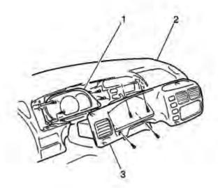
3. Remove the 4 screws (1) that hold the cluster in place.
