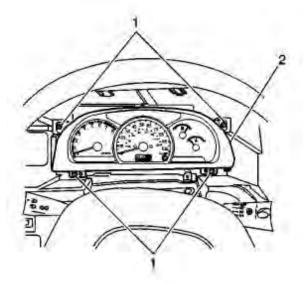
4. Pull the cluster forward to gain access to the electrical connectors
