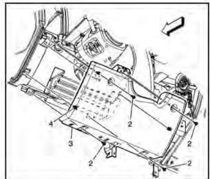
4. Remove the 6 screws retaining the bezel to the instrument panel (Chevrolet pic below).
